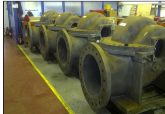
Pumps blasted and awaiting coating
