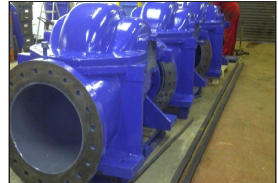
Coated pumps with ARC S2 inside and ARC S1 outside with UV resistant top coat
